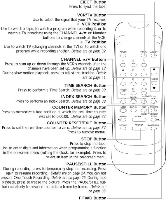
When tape playback is stopped, press to fast forward the tape at high speed. During tape playback, press to fast forward the tape while the picture stays on-screen. *Details are on page 35.* Press to add or delete channel numbers. *Details are on page 13.*
